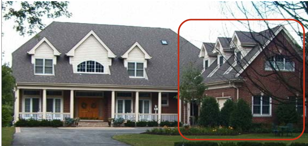
The garage is side loaded, with appropriately placed landscaping to de-emphasize the garage mass.
