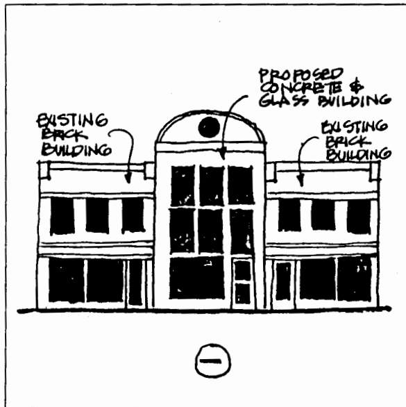
Figure 4-15 Relationship of Materials for In-Fill Construction
