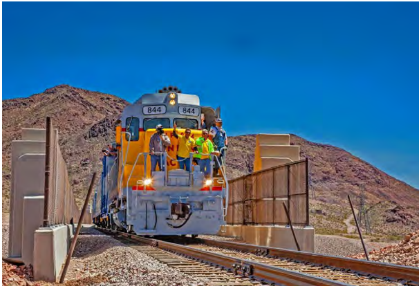
Representatives ride Union Pacific 844, an EMD GP-30 built in 1965 over the new bridge over Interstate 11 built to reconnect the Boulder City, NV's Nevada Southern Railroad Museum with Las Vegas. Photo credit: Frank Carroll, Nevada Southern Railroad Museum
