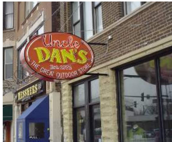
Internal illumination is not preferred and mounting hardware is not part of the sign design(4a2, 4b1)
